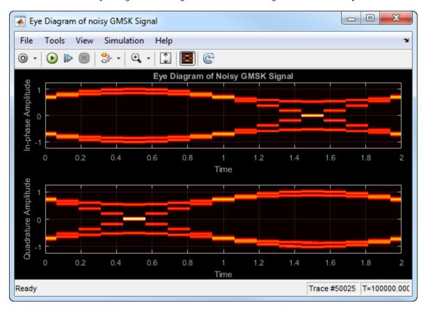
The lack of interpolation results in a plot having piecewise-continuous behavior.
