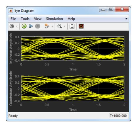
Open the configuration parameters dialog box. Change the  $\mathbf{Symbols}$   $\mathbf{per}$   $\mathbf{trace}$  parameter to 4. Run the simulation and observe that four symbols are displayed.
