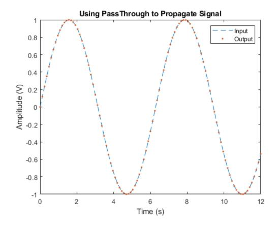
Verify the equality of input and output signals.
