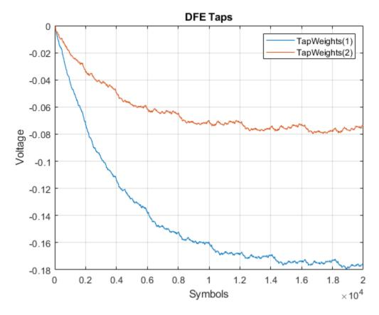
You can observe from the plot that the DFE adaptation is approximately complete after the first 10000 symbols, so these can be truncated from the array. Then plot the eye diagram by applying the reshape function to the array of symbols.
